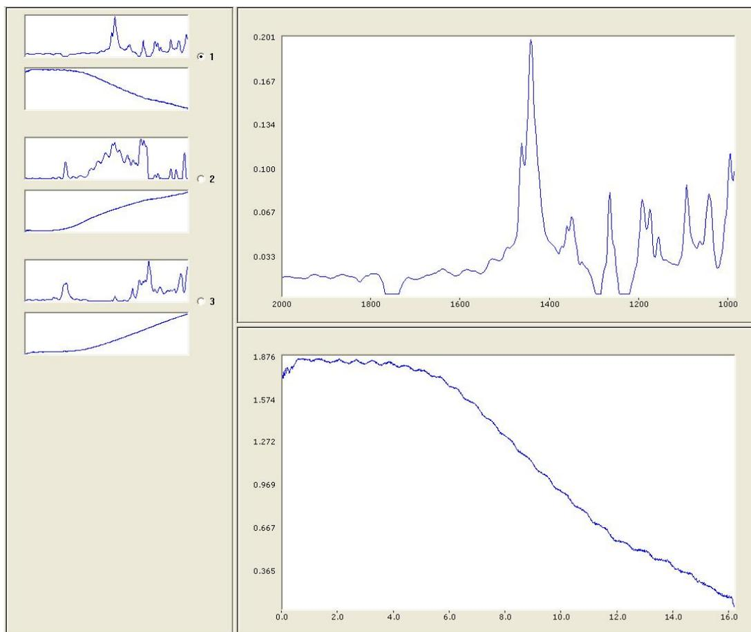
Remspec's ReactionSleuth™ software includes the ability to calculate “synthetic spectra” from complex data sets using a PCA/Target Transform method. The data from this reaction can be modeled successfully using three synthetic spectra, which are shown here with their calculated trend lines. The trace shown in the principal window matches the cyclohexene oxide starting material very well.
