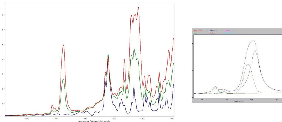
When the starting and ending spectra are overlaid with a spectrum from the middle of the reaction, it is clear that significant changes take place in the “fingerprint” region. In particular, an organic C=O feature near  $1740\text{ cm}^{-1}$  emerges as the reaction progresses. Close examination shows that this feature is not symmetrical. A peak-fit model can be built using two slightly displaced symmetrical peaks.
