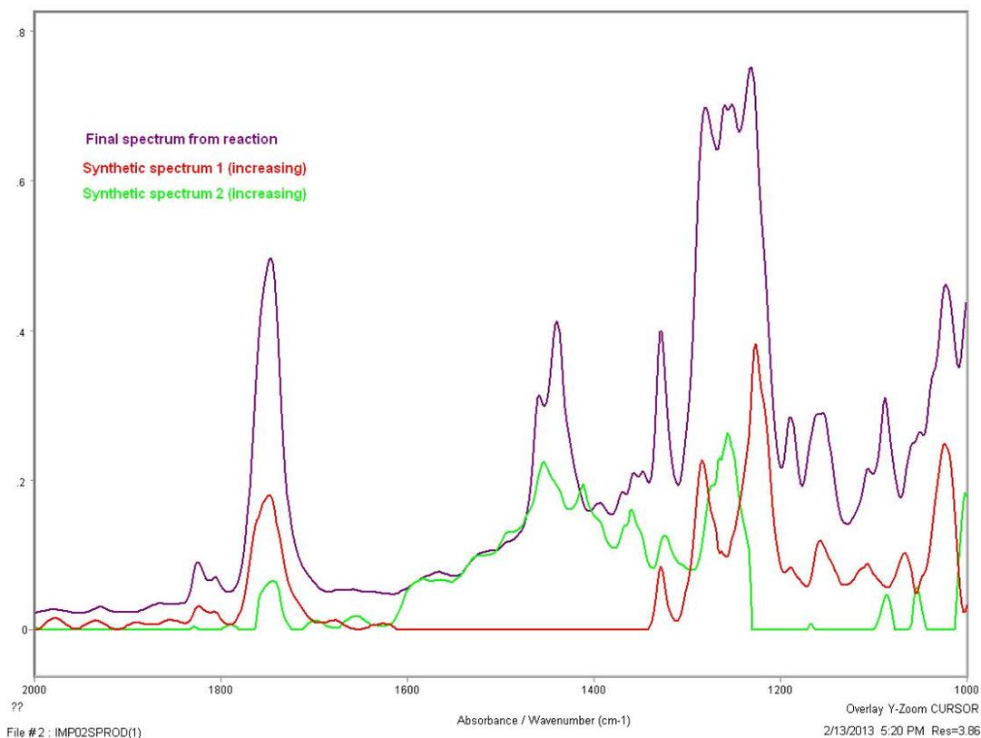
When the two synthetic spectra that have product-like trend lines are overlaid with the the final spectrum from the reaction, it becomes clear that the the reaction product spectrum is a mixture of the two synthetic spectra.
