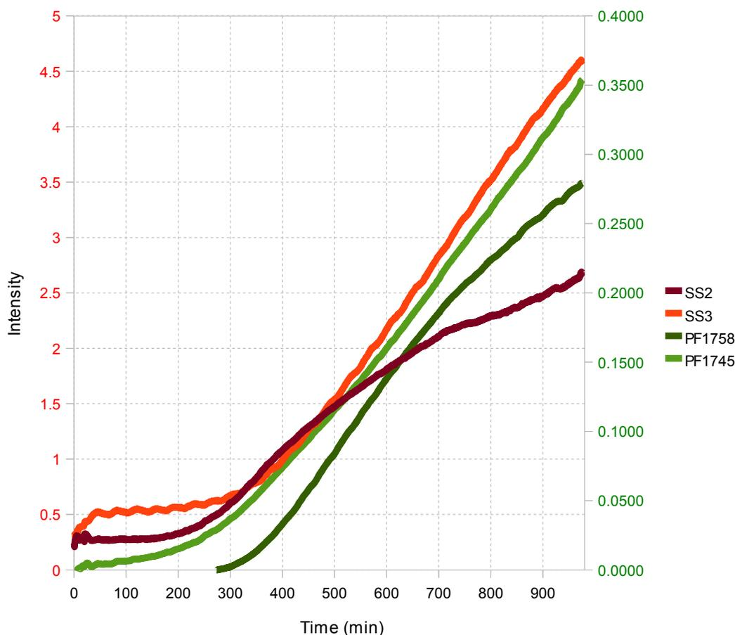
When we compare the “loadings”, or trend lines, for the synthetic spectra (SS2 and SS3 above) with the trend lines for the two carbonyl peaks that were modeled, some similarities are obvious. SS3 and the peak at  $1745\text{ cm}^{-1}$  both show essentially linear growth over time. SS2 and the peak at  $1758\text{ cm}^{-1}$  exhibit more complex behavior.
