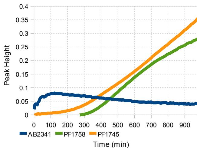
When the peak-fit model is graphed against time, it emerges that the two carbonyl peaks are associated with two slightly different reaction profiles. Here, they are displayed with a simple peak-height graph of the dissolved CO<sub>2</sub> peak in an autoscaled display.
