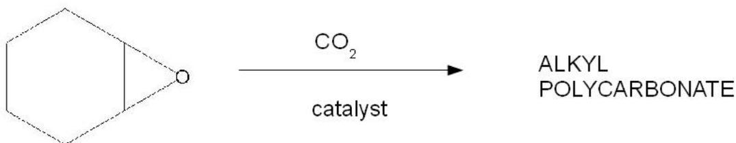
The manufacture of polycarbonates by polymerization of cyclohexene with carbon dioxide has been a topic of research for some time. The work described here uses a proprietary catalyst.  $\text{CO}_2$  was bubbled through the heated cyclohexene for 16 hours, and the reaction was monitored using a ReactionView system with a ZnS ATR crystal.
