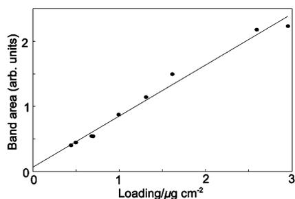
**Figure 7.** Plot of aspirin IRRAS band integral (1587–1618 cm<sup>-1</sup>) versus loading as determined by UV absorption colorimetry. Slope: 0.79 ± 0.04; Ordinate intercept: 0.21 ± 0.06; R<sup>2</sup> = 0.984.
