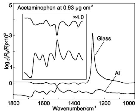
**Figure 3.** IRRAS (after correction for atmospheric  $\text{H}_2\text{O}$ ) of acetaminophen deposited at a loading of  $0.93 \mu\text{g}/\text{cm}^2$  on glass (upper trace) and aluminum (lower trace) coupons using the spray and smear methods, respectively.
