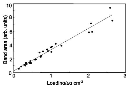
**Figure 6.** Plot of acetaminophen IRRAS band integral (1485–1527 cm<sup>-1</sup>) versus loading as determined by UV absorption colorimetry. Slope: 3.1 ± 0.1; Ordinate intercept: 0.2 ± 0.1; R<sup>2</sup> = 0.962.
