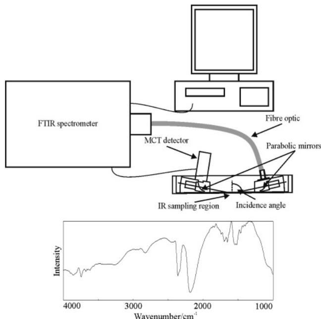
**Figure 1.** Schematic diagram of the instrument used for the measurement of the IRRAS of surfaces contaminated with organic compounds. (Inset) “Single beam” response of the system including the chalcogenide glass used in the fiber bundle.
