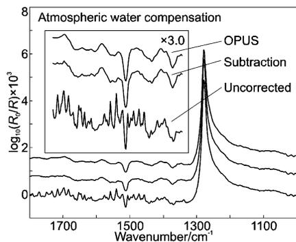
**Figure 2.** IRRAS of  $0.21 \mu\text{g}/\text{cm}^2$  acetaminophen on glass. (Lower Trace) Fine-structured spectral features above  $\sim 1400 \text{ cm}^{-1}$  due to atmospheric  $\text{H}_2\text{O}$ . (Middle and Upper Traces) Results of auto-subtraction of a reference  $\text{H}_2\text{O}$  spectrum and application of the Bruker OPUS atmospheric compensation, respectively. Both treatments reveal the underlying API bands.
