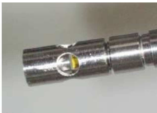
Figure 1: The liquid transmission head of a Remspec Mid-IR Fiber Optic Immersion Probe; the diameter of the head – and the probe shaft – is about 6 mm.
