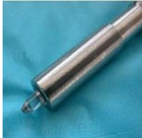
Figure 2: The TissueView ATR crystal is made of zinc sulfide and has a 1 mm diameter flat tip
